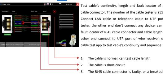
Test cable's continuity, length and fault locator of RJ45 cable connector. The number of the cable tester is 255. Connect LAN cable or telephone cable to UTP port of tester, the other end don't connect any device, can test fault locator of RJ45 cable connector and cable length. the other end connect to UTP port of wire receiver, enter
