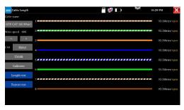
Note: The measured cable cannot be connected to any device. If connected to other devices, it will cause incorrect measurement results!
