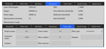
Measurement parameter includes laser wavelength, distance scope, pulse width, refractivity, back scattering coefficient, reflection threshold, bundling threshold, non-reflection threshold, and duration of measurement.
