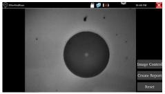
It is used to inspecting the cleanliness of the fiber end face
