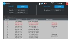
It is used for quickly find the IP address of the IP camera or other device connected to the instrument, supporting scanning MAC address, camera manufacturer, and scanning for IP conflicts.
