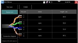
Connect cable to the LAN port of tester, the other end connect or disconnect other device. Enter "RJ45 cable TDR test" app to test cable's length. Test cable's length, please don't connect any device. The max measurement length is 600 meter.
